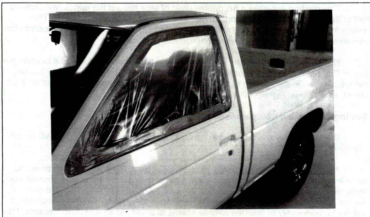
Figure 3-8 FULL DOUBLE LAYER OF TAPE ALONG ALL EDGES
